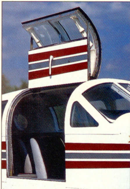
Dainty isn't the word you'd use to describe the Mustang's complex and heavy cabin door. Mooney thought it was a winner and patented the design. The generous elevator trim wheel and hefty gear lever dominate the center panel (left).
